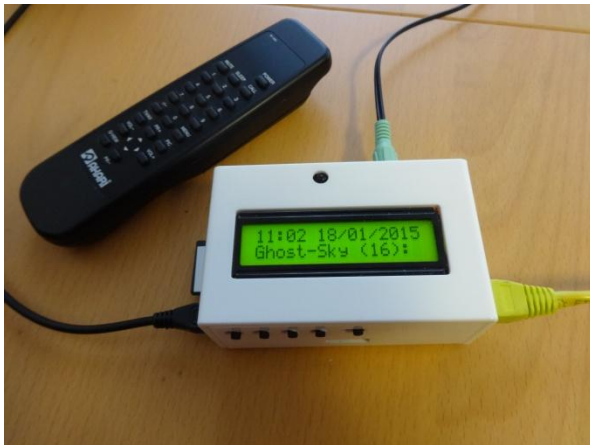
Figure 9 PiFace CAD Radio with IR Remote Control
