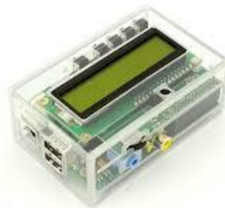
Figure 43 PiFace CAD in a case
