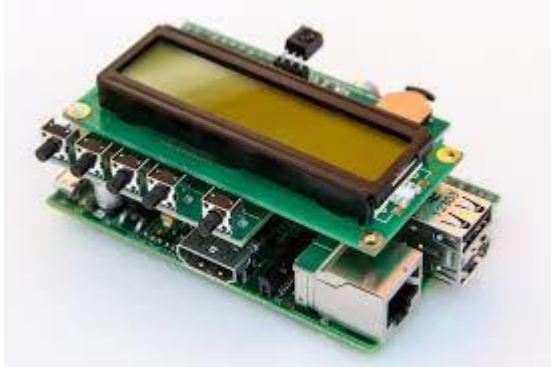
Figure 42 PiFace CAD and Raspberry PI
