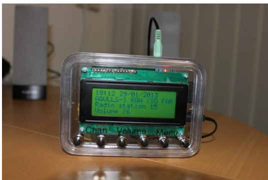
Figure 2 Four line LCD radio in a clear case
