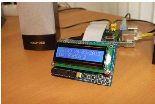
Figure 3 Radio using the Adafruit LCD plate
