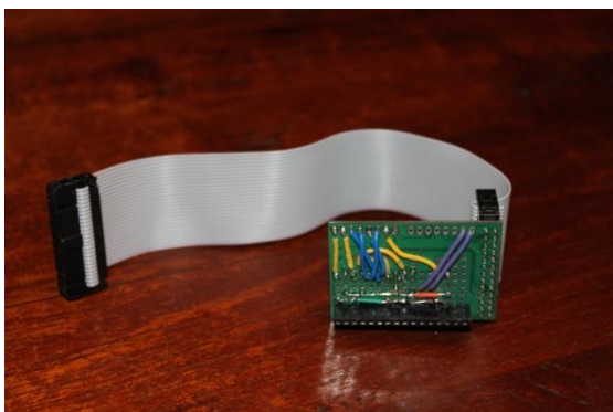
Figure 32 Interface board (Wiring side)
