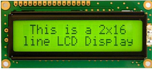
Figure 16 The HD44780 LCD display
