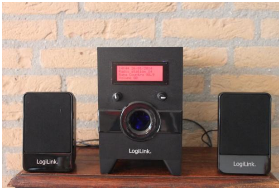
Figure 5 Pi radio using rotary encoders
