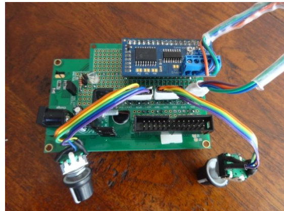
Figure 41 The I2C backpack interface board
