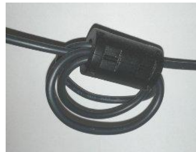
Figure 25 Loop +5V supply around the core
