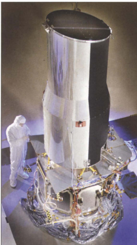
Just chill. SIRTF's silver and black coatings will reflect solar heat and radiate the telescope's heat, respectively. (Solar panels are not shown.)
