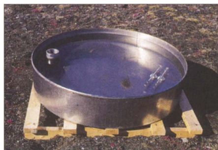
Installations of the water evaporation pan. (Left) A Canadian Class-A pan installed at the northernmost point on Earth where evaporation pans were used (79°25'N, 90°45'W). The pan is separated from the ground with a wood plank to avoid local effects from the ground. (Right) A Chinese pan at Hongwuyue, Tenshan Mountains. The pan is buried in an effort to minimize the effect of the exposed side wall.
