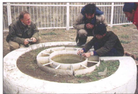
Installations of the water evaporation pan. (Left) A Canadian Class-A pan installed at the northernmost point on Earth where evaporation pans were used (79°25'N, 90°45'W). The pan is separated from the ground with a wood plank to avoid local effects from the ground. (Right) A Chinese pan at Hongwuyue, Tenshan Mountains. The pan is buried in an effort to minimize the effect of the exposed side wall.
