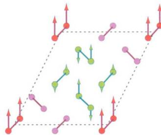
**Complex order.** In the magnetization plateau of  $\text{SrCu}_2(\text{BO}_3)_2$ , with a net magnetization of  $1/8$  of the saturation value, the spins of the  $\text{Cu}^{2+}$  ions form a complex pattern: one in eight of the dimers are strongly polarized parallel to the magnetic field, whereas the remaining dimers have a weaker staggered polarization.
