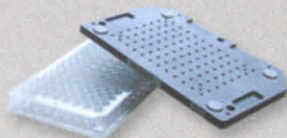
Illumina's 96-bundle Sentrix™ Array allows parallel processing of over 150,000 SNPs.
