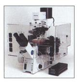
ing the light path from eyepiece to cameras at the back or left side ports, and shutter exchange between fluorescence and transmitted light. A universal condenser for brightfield, phase contrast, and differential interface contrast observations is motorized to change optical components and aperture settings.
