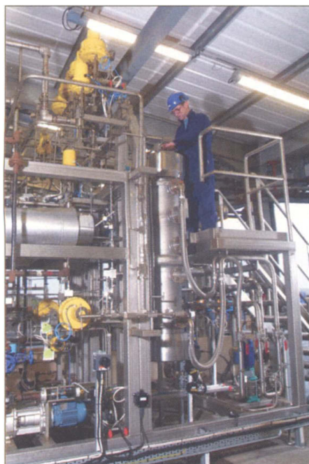
Fig. 1. Part of the multipurpose plant at Consett, Co Durham, United Kingdom, for chemical manufacture in supercritical \text{CO}_2 . The plant is a good example of a green technology, developed in a university, being evaluated on a commercial scale in industry. More such trials are needed to implement new green chemical technologies. [Photo courtesy of Thomas Swan & Co. Ltd.]
