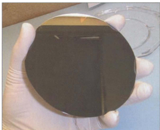
Fig. 5. A silicon wafer coated with a 193-nm photoresist system using a liquid CO 2 spin coating tool operating at slightly below room temperature. [Provided by the NSF Science and Technology Center for Environmentally Responsible Solvents and Processes: (67)]
