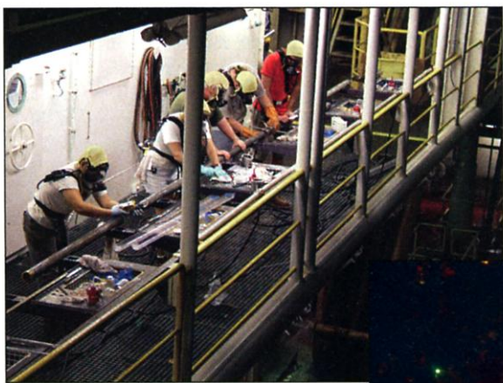
Smelly work. Processing ocean sediment cores onboard JOIDES Resolution can require respirators for the mud’s hydrogen sulfide, but it can yield slow-living microbes (right, green dots) from 30 meters deep.
