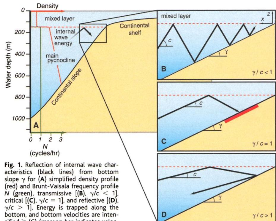
**Fig. 1.** Reflection of internal wave characteristics (black lines) from bottom slope  $\gamma$  for (A) simplified density profile (red) and Brunt-Vaisala frequency profile  $N$  (green), transmissive [(B),  $\gamma/c < 1$ ], critical [(C),  $\gamma/c = 1$ ], and reflective [(D),  $\gamma/c > 1$ ]. Energy is trapped along the bottom, and bottom velocities are intensified in (C) (maroon bar indicates velocity intensification); bottom velocities also increase upslope in (B) (10).
