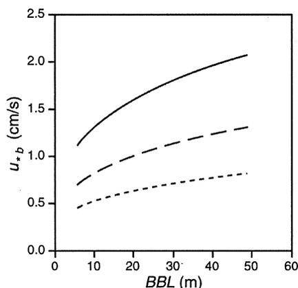
**Fig. 4.** Bottom velocity shear  $u_{*b}$  plotted against thickness of bottom boundary layer (BBL)  $h$  using Eq. 2. Solid, long-dashed, and short-dashed lines indicate  $u_o = 20, 10,$  and  $5$  cm/s, respectively.
