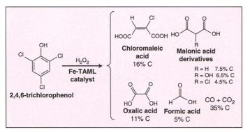
**Efficient oxidation.** The new catalyst described by Sen Gupta *et al.* breaks up the persistent pollutant TCP into smaller, acyclic products, which can be consumed by microorgranisms. The catalyst shows similar activity for another persistent pollutant, pentachlorophenol.
