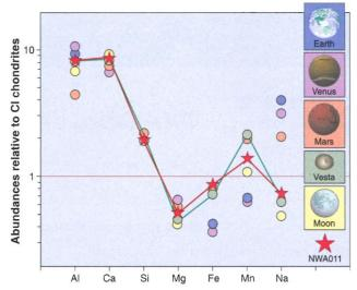
**Similar, but not the same.** The major element compositions of basalts from Earth, Venus, Mars, Vesta, and the Moon are compared to that of the new basaltic meteorite, NWA011 (4). The patterns for Al, Ca, Si, and Mg are remarkably similar. Low Fe in terrestrial basalts indicates a large core. Large variations in Na reflect differences in initial volatile element inventory. NWA011 data from (1), all other data from (5).
