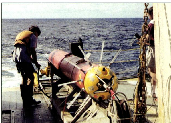
No swizzle stick. This turbulence sensor helped show that salt fingering, not stirring, was mixing tropical waters.
