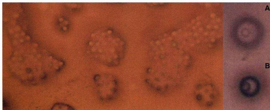
**Fig. 4.** Collection of near monodisperse capsules. Magnified views of two capsules formed under different parametrical conditions are also given in the figure. In (A), the outer diameter is  $10 \mu\text{m}$ , whereas the diameter of the capsule shown in (B) is  $8 \mu\text{m}$ . The hardening process can also be thermally or chemically initiated under the use of appropriate reagents.
