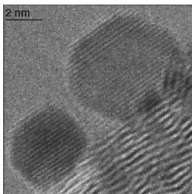
**Fig. 2.** Representative in situ TEM image of the unpromoted Ru catalyst recorded at a temperature of  $331^\circ\text{C}$  and a pressure of 3.0 mbar in a gas composition  $\text{H}_2/\text{N}_2$  of 3:1. No surface features are seen on any of the Ru crystals. The lattice spacing is 0.21 nm corresponding to the (101) planes. The Ru crystals show well-developed facets.
