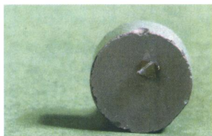
Fig. 2. Flux-grown octahedral crystal of \text{Ho}_2\text{Ti}_2\text{O}_7 stuck to a NdFeB permanent magnet at room temperature. The strong paramagnetism reflects the large magnetic moment of \text{Ho}^{3+} .
