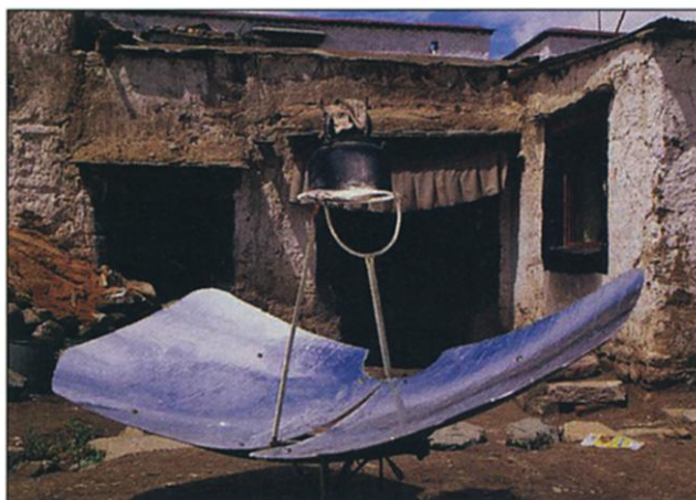
Diffusing technologies for concentrating energy. The use of solar cookers, such as this parabolic concentrating type that has been widely distributed in China, can reduce the environmental and health effects of collecting and burning biomass resources.
