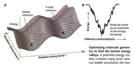
est of which is the global minimum (the most stable structure). The minima differ by rotations about single bonds. The potential energy surface shown here illustrates two degrees of freedom, but real molecules may contain degrees of freedom on the order of tens to thousands.
