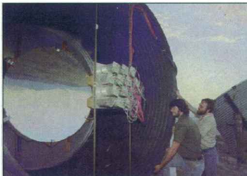
Catching mystery rays. A prototype detector at the Fly's Eye in Utah, which is searching for the highest energy cosmic rays.
