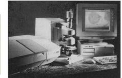
metals; and Micro-ATR mode for black rubbers, filled polymers, and paper. A variable aperture allows the ability to mask down onto a sample to the diffraction limits of 10 by 10  $\mu$ m. Permanently aligned optics enable high-performance, no-alignment operations, making sample identification possible in seconds.
