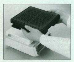
four microtiter plates or two culture flasks at one time. It features a nonskid surface and is 225-mm square.
