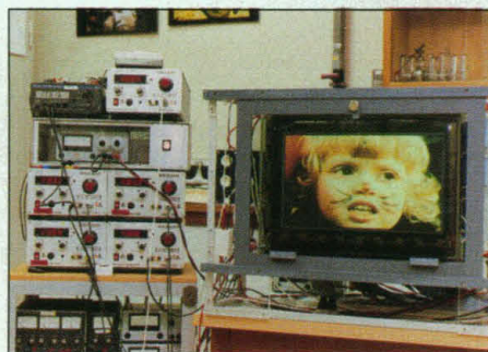
Making screens skinny. A trimmed-down conventional CRT (above) is one route to a flat-panel display; another uses an array of nanotips like the one coupled to a gated transistor (top right).
