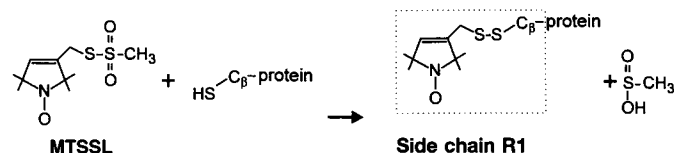
Fig. 2. Reaction of spin label to generate nitroxide side chain R1.
