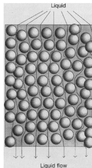
**Fig. 7.** Schematic view of the flow of a liquid through a bed of uniformly sized beads.
