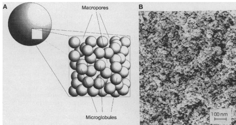
**Fig. 2.** (A) Schematic view of the morphology and (B) scanning electron micrograph of the internal structure of a macroporous polymer bead.
