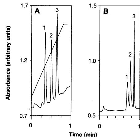
**Fig. 10.** Fast separation of (A) proteins by reverse-phase chromatography in a gradient of acetonitrile in water and of (B) polystyrene standards by precipitation-dissolution chromatography in a gradient of tetrahydrofuran in methanol on a 50-mm-long molded poly(styrene-co-divinylbenzene) column with an 8-mm inside diameter. Proteins: cytochrome c (1), myoglobin (2), and ovalbumin (3); polystyrenes: molecular weight 9200 (1), 34,000 (2), and 980,000 (3).
