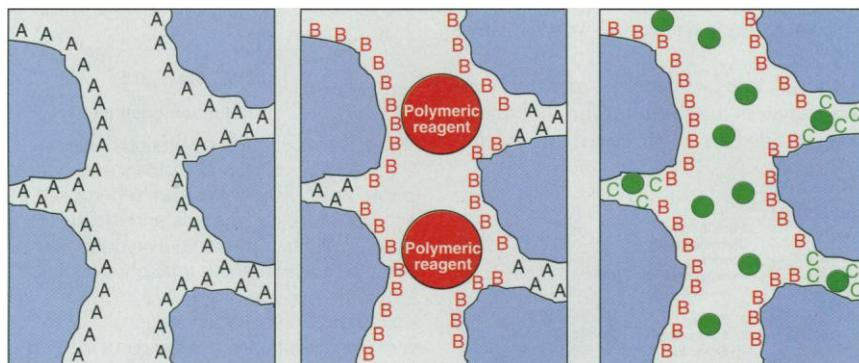
**Fig. 5.** Concept of pore size-specific functionalization of macroporous polymers. The large polymeric reagent transforms those functional groups A that it comes into contact with (those in large pores only) into B, and the small reagent transforms all remaining functional groups (those in small pores) into C.
