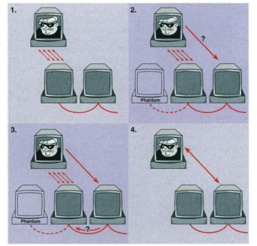
**Diversionary tactic.** In a common strategy called network intrusion, a hacker floods one computer with messages (1), then requests entry from a second computer while posing as a legitimate part of the network (2). The second computer asks the first to authorize the connection (3). The first computer is too overwhelmed to respond, so the second computer accepts the request, and the hacker gains access to the system (4).
