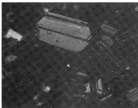
Fig. 2. Optical micrograph of \text{K}_1\text{C}_{60} single crystals embedded in a microcrystalline matrix (size 340\ \mu\text{m} by 500\ \mu\text{m} ).
