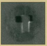
The shadow knows. "Transillumination" images of a T-shaped block of rubber immersed in an opaque fluid; a three-dimensional image computed from them is shown at bottom.
