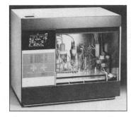
Operating parameters such as media flow, pH, dissolved oxygen, and temperature are continuously monitored and controlled, with oxygen consumption rate calculated on-line as medium directly perfuses across the culture. Integra Biosciences/Tecnomara. Circle 144.
