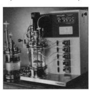
interactive four-gas control system regulates pH and dissolved oxygen. The BioFlo 3000 is available with a variety of vessel types and impeller designs, including a unique packed basket capable of producing animal cells to 108 cells per cubic centimeter of basket volume. New Brunswick Scientific. Circle 94.
