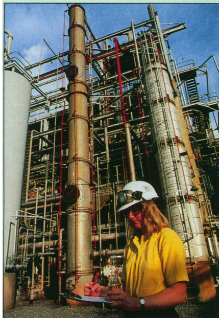
Taking responsibility. Equipment that recovers cyclohexane, a volatile industrial solvent.
