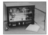
by 150 mm hybridization bottles simultaneously. The unit features a small footprint, simple digital controller, and a stackable design that allows for two ovens to be run simultaneously at different temperatures. Integrated Separation Systems. Circle 94.
