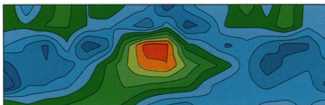
Fig. 2. A two-dimensional image created by seismic tomography shows long wavelength features of the structure including a broad low-velocity region, much larger than the extent of the bright AMC reflection, that may contain a part liquid/part solid crystal mush. Image shows a region 6 by 16 km. [Adapted from (12)]
