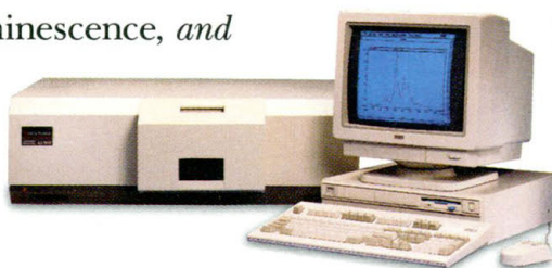
The Model LS-50B Luminescence Spectrometer is PC-controlled with Fluorescence Data Manager Software.
