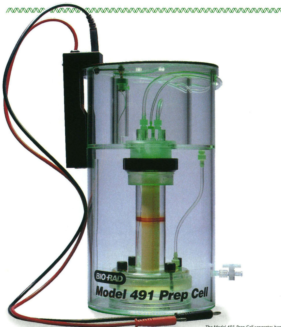
The Model 491 Prep Cell separates hemoglobin A (pI 7.1) from hemoglobin C (pI 7.4). Both molecules have identical mass-64.5 kd. Native-PAGE was performed using Tris-CAPS electrophoresis buffer (pH 9.4).
