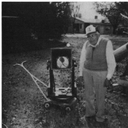
"Portable telescope mounted on a lawnmower chassis. Photo courtesy of Dr. Clyde Tombaugh. Note the curved secondary mirror holder which minimizes the apparent effects of the diffraction spikes." [From Unusual Telescopes ]
