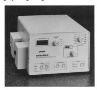
other attenuating optics. A prealigned longlife deuterium lamp is used for the ultraviolet region. For performance at wavelengths above 360 nm, a prealigned tungsten lamp is available. Rainin Instrument Co. Circle 80.
