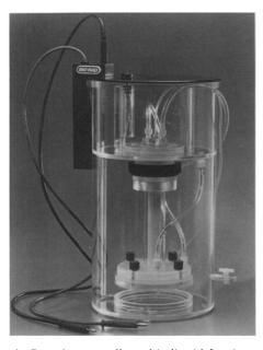
sis. Proteins are collected in liquid fractions for immediate use in subsequent characterization and assay procedures. The unit is useful for purifying proteins for use in se-
