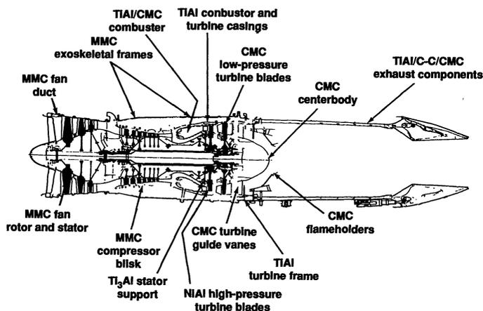
**Fig. 4.** Cross-sectional view of an advanced turbine engine showing the applications for advanced materials technology. Abbreviations: MMC, metal matrix composite; CMC, ceramic matrix composite; and C-C, carbon fiber in carbon matrix.
