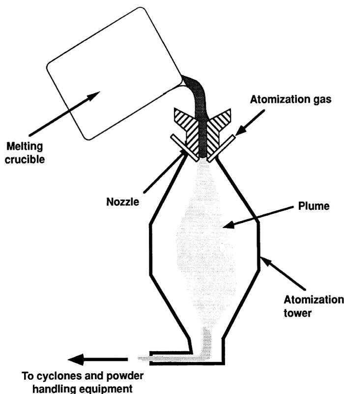
**Fig. 3.** A schematic representation of a gas atomizer used to produce superalloy powders.
