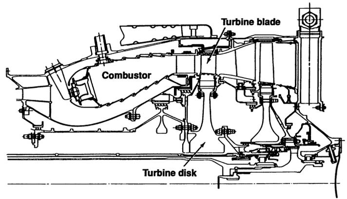
Fig. 1. Cross-sectional view of an F404 gas turbine engine showing the combustor and turbine hot section components.
