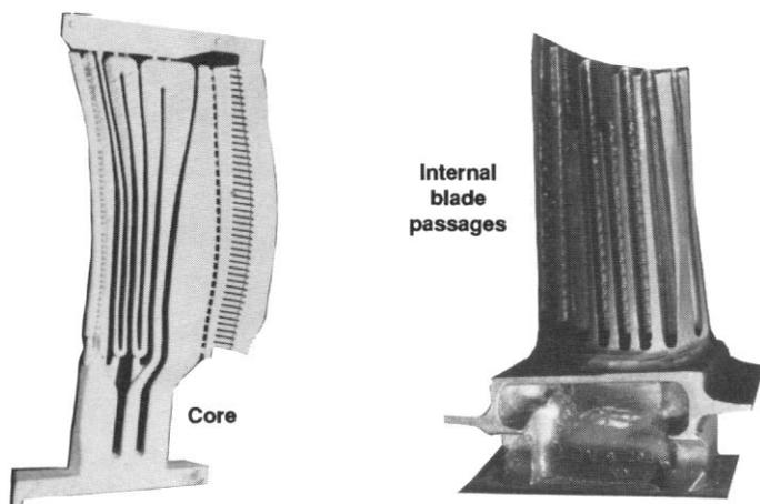
**Fig. 2.** Typical core (left) used to produce internal turbine blade cooling passages during investment casting. The turbine blade (right) has been machined to show the internal passages.
