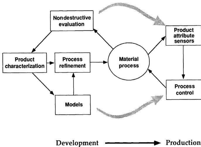
**Fig. 5.** Modern materials processing uses advanced sensors, process models, and control technology to provide consistent high-quality material. This strategy permits knowledge and expertise to transfer from the development laboratory to the factory floor more efficiently and quickly.
