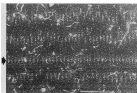
Fig. 6. Decoration of a face parallel to the c axis on the edge of a YBCO crystal at a field of 8 G. The arrow marks a twin boundary and is also the c direction. Note the oval vortices [from (24)].
