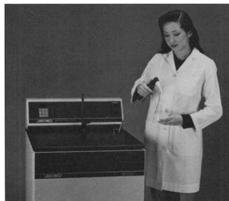
also available. All filters and membranes are housed in a completely assembled compact cabinet with epoxy-coated steel front and sides. A feedwater line, drain line, and electrical outlet are the only connections required for operation. Two kinds of water are delivered at a rate of up to 1.6 liters per minute: laboratory grade water provided via reverse osmosis to a gooseneck faucet and Type I reagent grade water through a polishing unit to a dispensing gun. Labconco. Circle 326.
