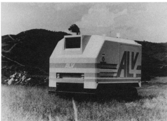
Fig. 6. The Autonomous Land Vehicle, a project sponsored at Martin Marietta Corp. by the Defense Advanced Research Projects Agency (DARPA). The vehicle carried TV cameras and computers, and drove itself along a road network using information about road geometry derived from the TV images.
