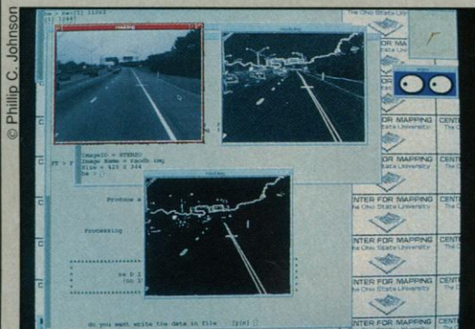
The thin white line. A mapping computer locates the edge of the road in a video image.
