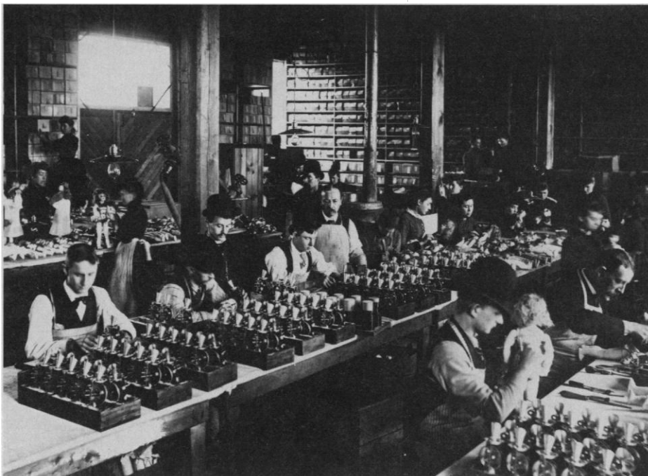
Manufacture of talking dolls in Edison's Phonograph Works, about 1890. "With [his] dictating machine in trouble, Edison looked to the doll to keep the business afloat. . . . There was nothing wrong in the marketing strategy; the talking doll proved to be so popular that orders soon out-stripped supply. The problem was in the small phonograph movement inside the dolls. The diaphragm/stylus assembly simply would not stay in the fine groove of the wax record. Consequently most of the dolls failed to work properly, steadfastly refusing to talk for their owners. One dealer reported that 188 dolls were returned out of 200 sold." [From Edison and the Business of Innovation ]
