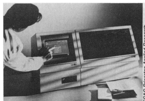
Low-level light detector. The OMA III Model 1433 by EG&G Princeton Applied Research is a cryogenically cooled charge-coupled device array detector to record extremely low light level, two-dimensional spectral images, for use in Raman spectroscopy, fluorescence, and emission spectroscopy.
