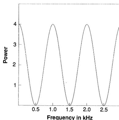
Fig. 1. Spectral density function for  $n(t) + n(t-\delta)$ , where  $n(t)$  is a band-limited (0 to 3 kHz) Gaussian noise, and  $\delta$ , the delay parameter, equals 1 ms.
