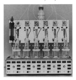
ent; these parameters include dissolved oxygen, pH, air flow rate, and agitation speed. Included with the Micro-Jar Fermentor are a peristaltic pump, an air-flow meter, a digital temperature display, and a digital agitation-speed display for each jar. Xyferm-Filenco, a Division of JSJ Manufacturing. Circle 497.
