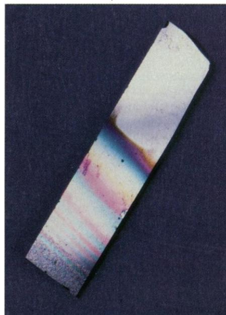
Fig. 1. Diamond(111) film epitaxially grown on room temperature Si(111) from 120-eV mass-selected C<sup>+</sup> ion beam. The color interference fringes are the result of the varying thickness profile of the film. The maximum thickness is on the side where the fringes converge; the number of fringes indicate a thickness of ~7000 Å in that region.
