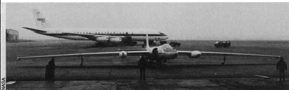
Two ways to sniff out ozone-destroying chlorine. The ER-2 research plane (foreground), a modified version of the U-2 spy plane, flies high with its lone pilot and computerized instruments to make insitu measurements while scientists man the DC-8 to make many remote observations.
