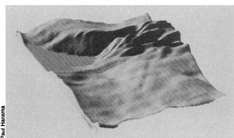
down to keep the current constant. By recording the ups and downs of the tip as the probe moves over the surface, the SICM constructs a topographic map of the sample.
