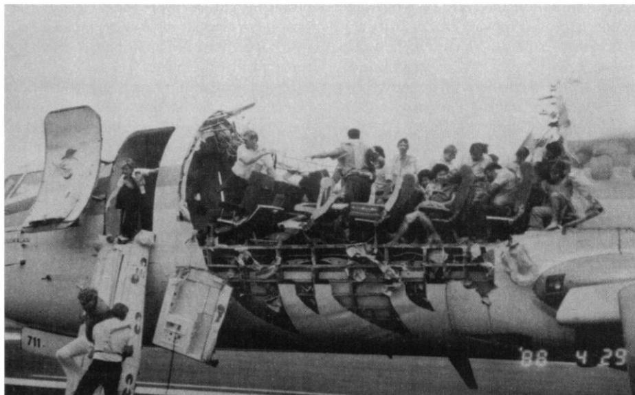
Coming apart at the seams? A 19-year-old Boeing 737 split apart last April along a weak skin splice that had been the subject of concern since 1972.
