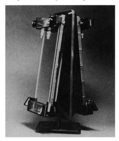
tank's silicon gasket to compress against the glass plate, forming a leakproof seal. Both the upper and lower buffer tanks can be removed for cleaning and decontamination. To reduce smiles, the gel is sandwiched between a treated glass plate and a glass plate coated with a thermoconductive material. The Base Runner Sequencer has a footprint of 36.2 cm<sup>2</sup>. International Biotechnologies. Circle 544.
