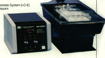
I-C-E System includes isoelectric focusing cover with adjustable platinum electrodes and buffer tanks for 1D and 2D separations.
