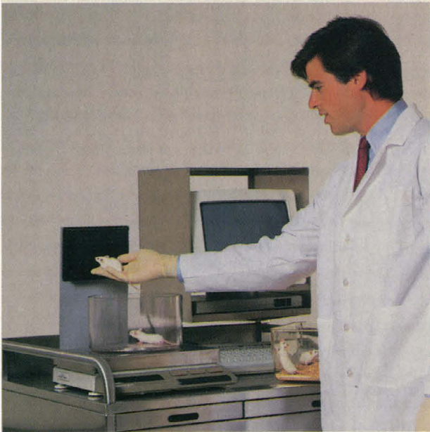
The animal is identified as it passes near the stationary reader.
